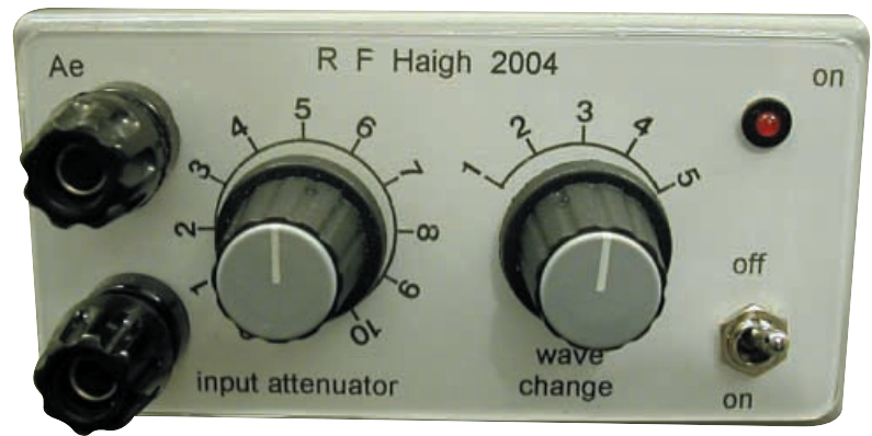
Layout of components and lettering of components mounted behind the top of the Receiver case. This arrangement allows room for a slow-motion drive for a front panel dial
